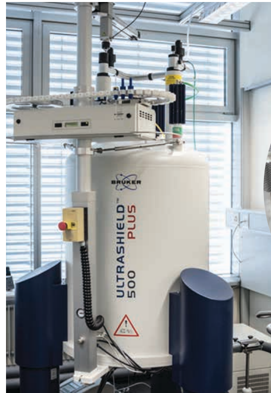
Microprobe NMR instrument for structure analysis.
