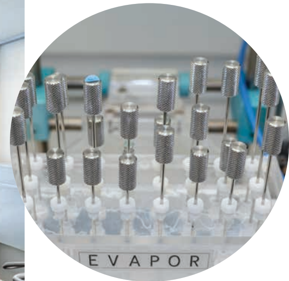
Small scale evaporation of active extracts.
