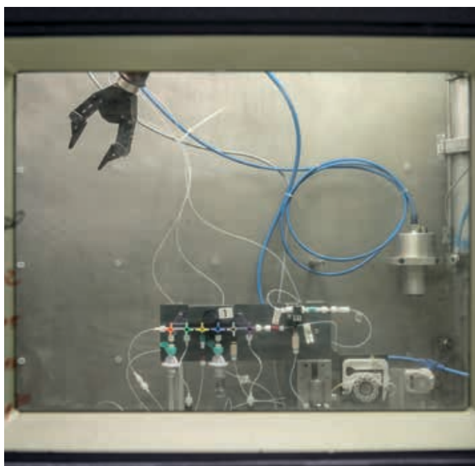
Chemical separation system for Tb radionuclides.
